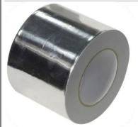
FDP3107 is a single sided aluminium foil with a water based acrylic adhesive and a siliconised kraft release liner. The 100 Micron conformable, aluminium foil is very durable and has excellent properties including resistance to moisture vapour transmission. Benefiting from very high shear resistance and high peel adhesion, the relatively slow rate of bond development allows repositioning for some time after contact on most substrates.
