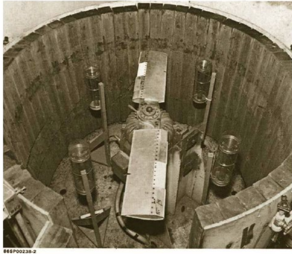
Picture 2.3-1; Picture of Boeing M&PT Rain Erosion Test Fixture
