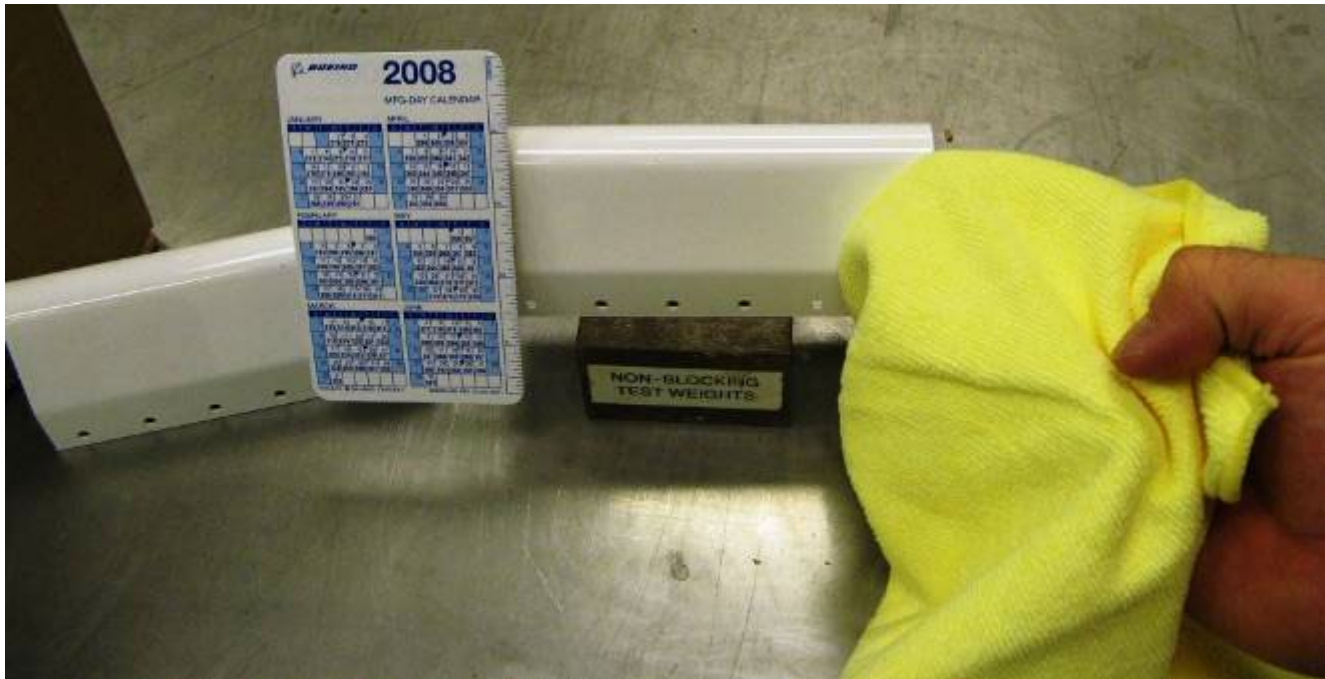
Picture 1.2-1; Example of Paint Sealant Application to Rain Erosion Foils
