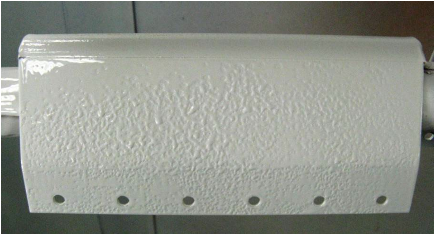
Picture 1.5-1; Typical Example of Secondary Topcoat De-wetting When Applied over Topcoat with Paint Sealant Applied
