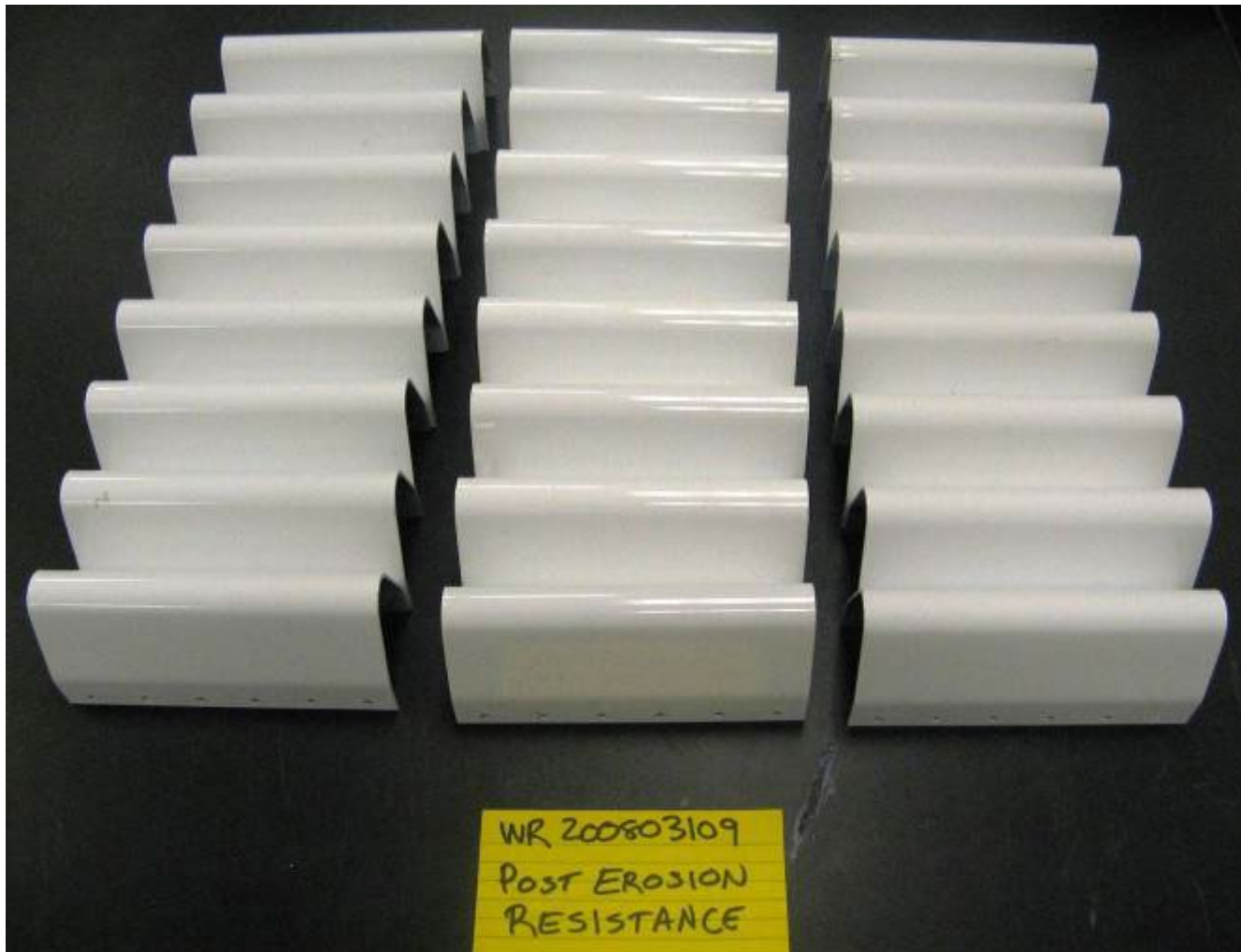
Picture 2.3-2; All Painted and Sealant-Treated Rain Erosion Foils Following Rain Erosion
