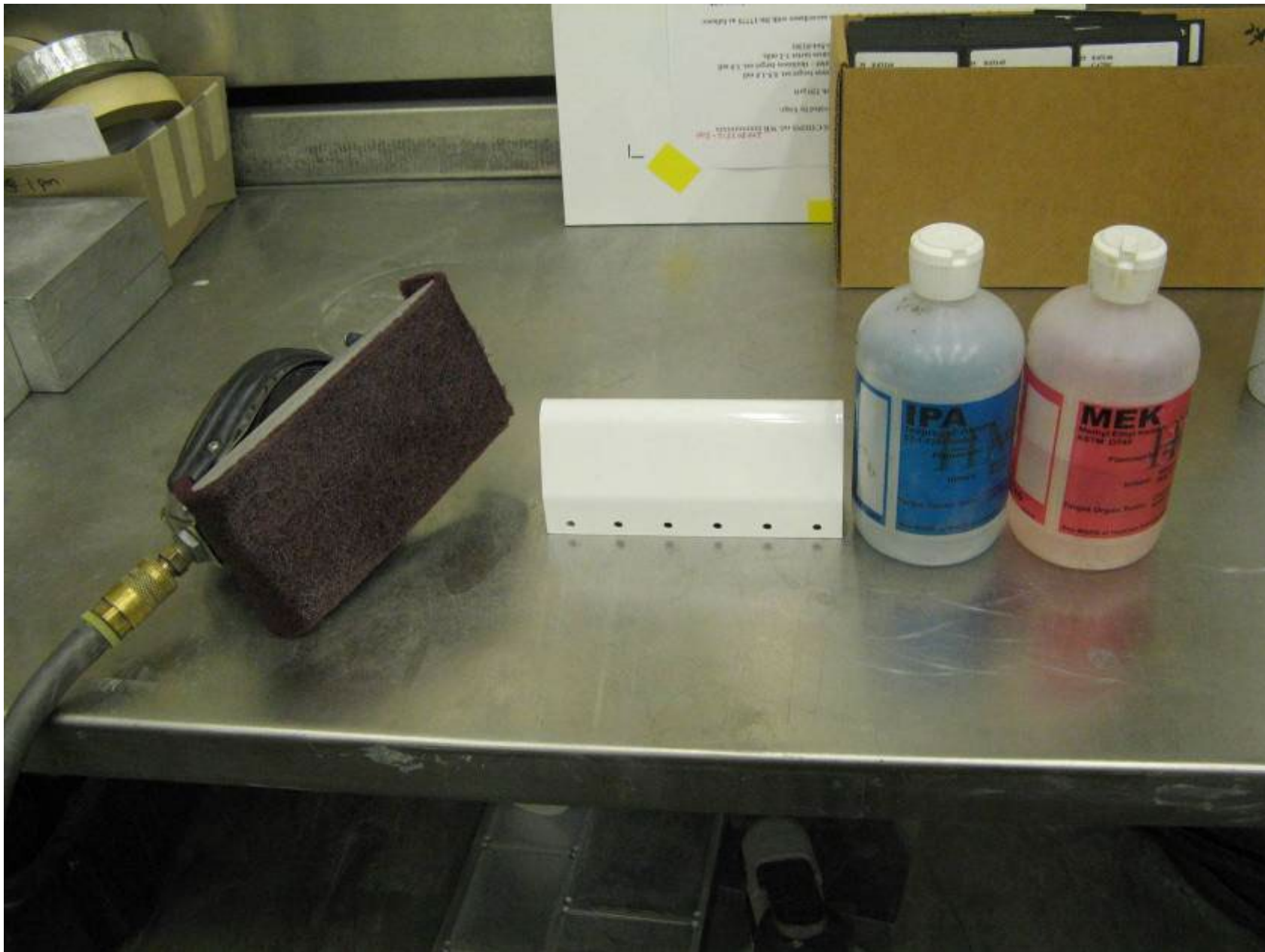
Picture 1.3-1; Example of Topcoat Reactivation and Paint Sealant Removal On Rain Erosion Foils
