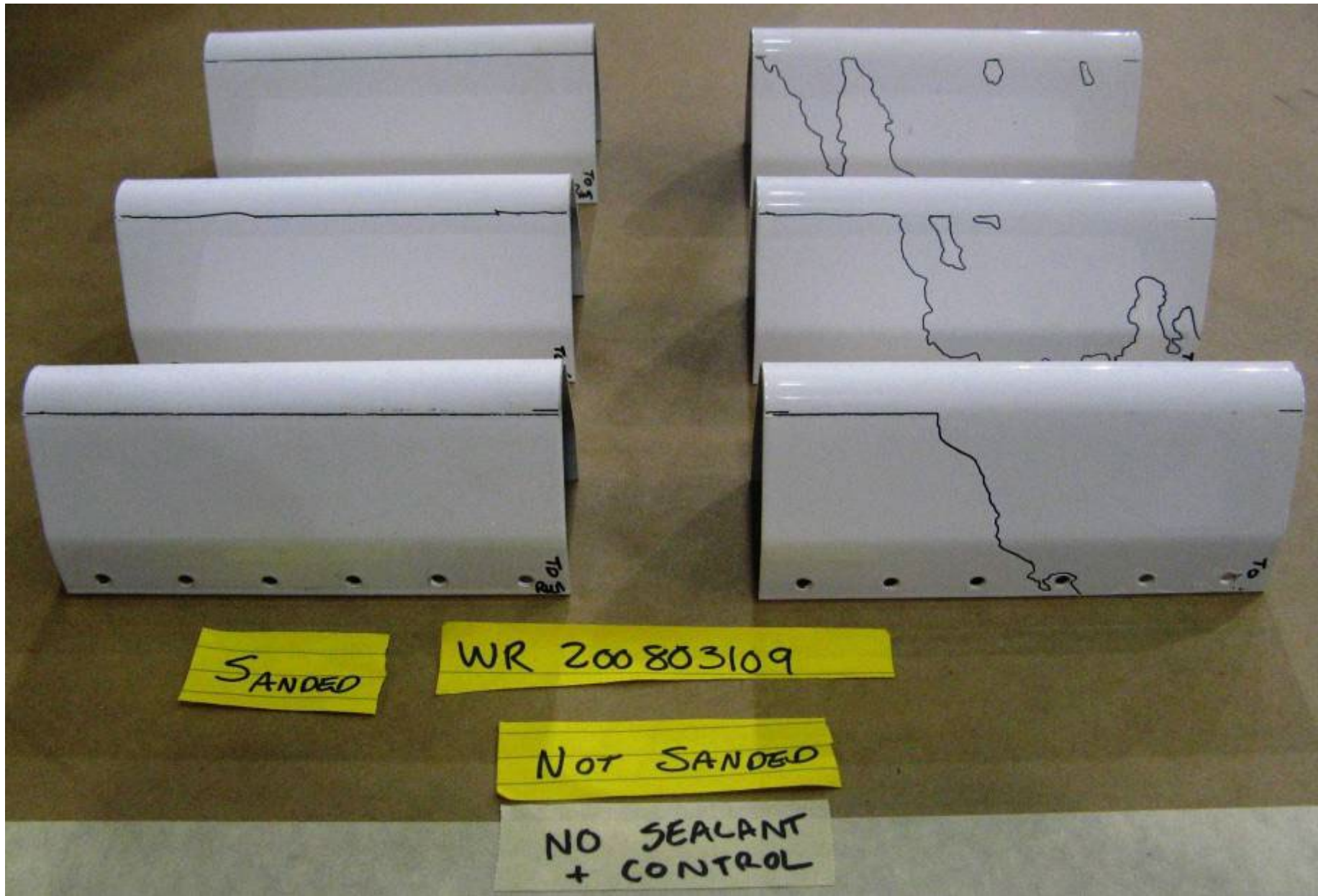
Picture 1.5-4; Post Rain Erosion, Overcoat Adhesion, No Paint Sealant, Control Foils
