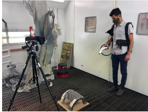
Figure 3: A sample is stretched over a curved surface on the ground, and sprayed at 45°
