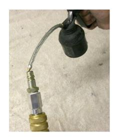
Apply two drops of air tool oil to the rear of throttle daily.
