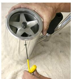
Loosen gear unit using a 41 mm wrench, turning clockwise (left handed threads).
