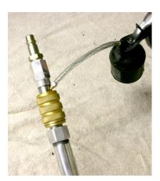
Apply three drops of air tool oil in the groove of the throttle body daily.
