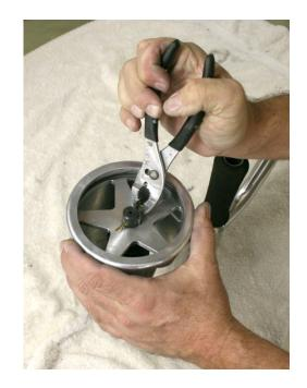
Remove the drum by loosening the 3/32 set screw using t-handle allen wrench  $\frac{1}{2}$  turn.
