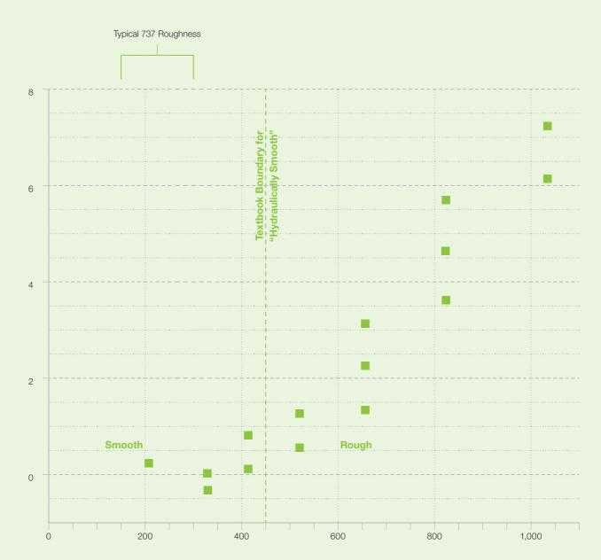
Equivalent sand-grain size, in microinches, on wing supersonic "rooftop."
